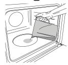
Only when the oven is cold, fill the embossing of the cavity with the quantity of drinking water suggested in the relative cooking table. Place the food in the oven. Set and activate the steam function: At the end, carefully open the door and let steam escape slowly.
