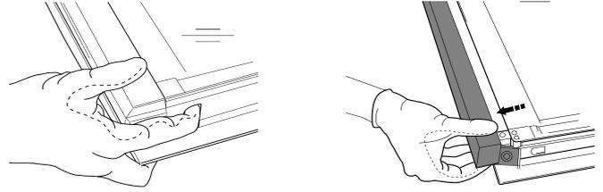
**2.** Lift and firmly hold the inner glass with both hands, remove it and place it on a soft surface before cleaning it.
